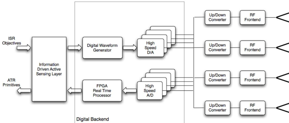
**Figure 1: Multi-mode, Multi-channel Software-Defined Radar**
